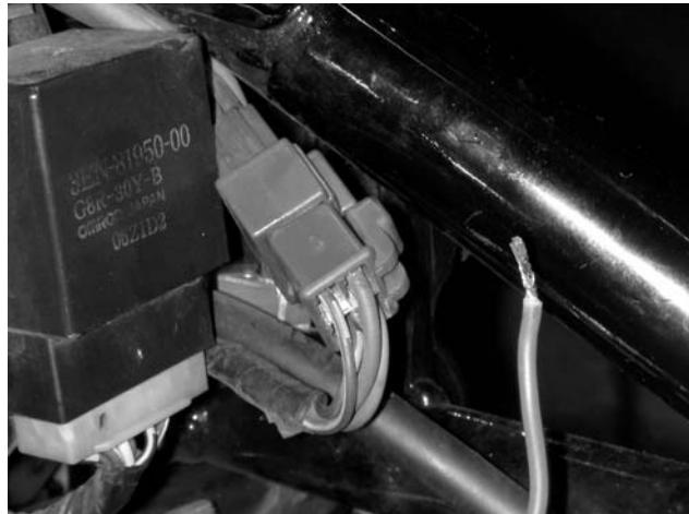
You can see the ‘hot’ wire for the cigarette lighter here. I inserted it just under the hot lead in the above block with a spade lug, some dielectric grease, and a little electrical tape to protect the wire.
