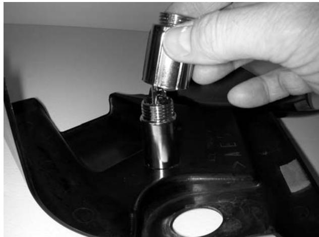
When you are satisfied with the fit, and have the weather proof cap of the lighter rotated to the angle you want it (I had the cover on top, to lessen the likelihood that it would fall out) then you can secure the lighter by screwing the outer sleeve in place and, if you like, adding some cement to the inside for good measure. I used "Pit Crew's Choice" which secured the lighter nicely.
