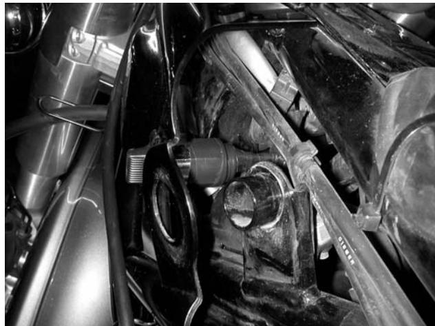
It is a bit of work to get the two neck covers to hook up at the top (the “gull wing” thing again), before making sure their large holes go over the fuel tank bumper pipes. Check as you go that the wires don’t bind or pull loose.
